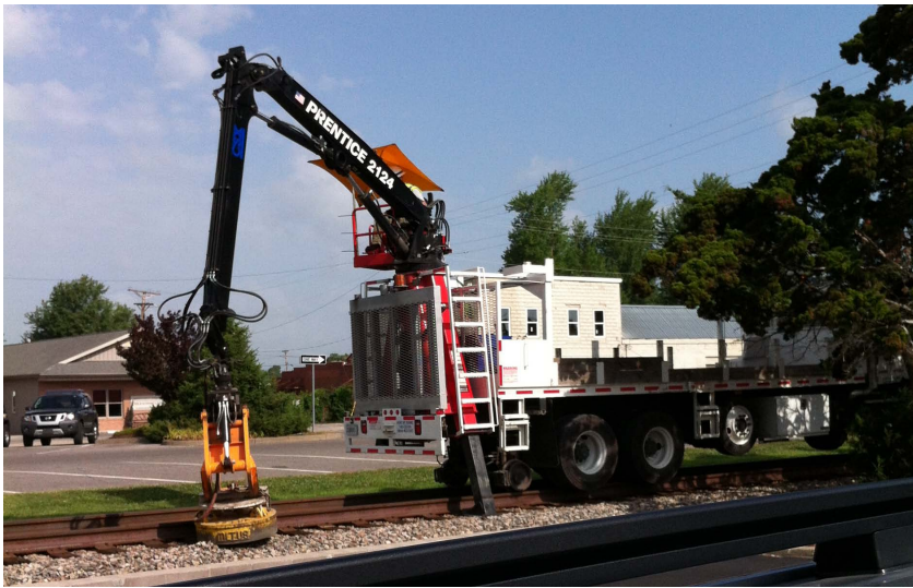
Above: A specialized magnet truck clears metal along track right-of-way in downtown Madisonville. -Bill Corum
