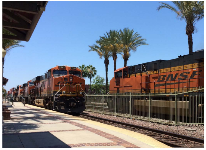
A meet between two stack trains at Fullerton Station. The train on track three, closest to the platform, has a hold order to wait for one more train before advancing on track two to continue east towards San Bernardino, CA.
